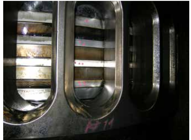
Minimal deposits and wear on a piston ring in a MAN B&W 12K98ME-C7.1-TII engine with more than 6,000 running hours using Shell Alexia 50.
